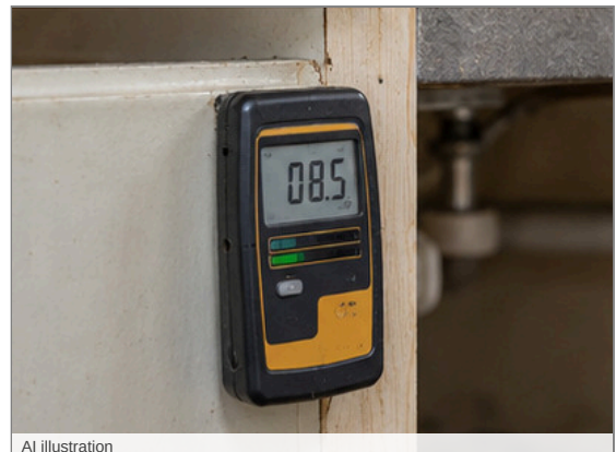
Photo - 109 Low moisture reading
